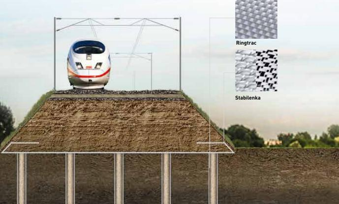
Activation of high circumferential tensile forces and radial support
