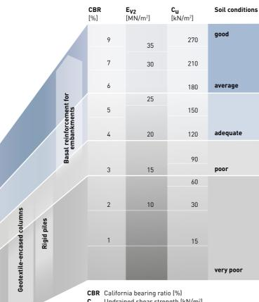
Undrained shear strength (kN/m<sup>2</sup>) Cu Ev2
