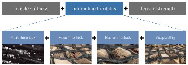
Rough surfaced geogrids achieve microscopic interlock with soil particles (friction)
