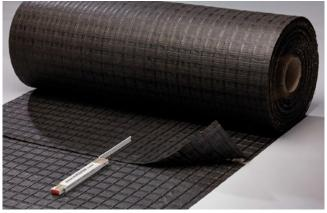
In the length direction the jointing of the rolls should be with a 250 mm overlap. The end of a roll should always be placed over the beginning of the next, ensuring the overlap is not lifted during the asphalt covering operation.
