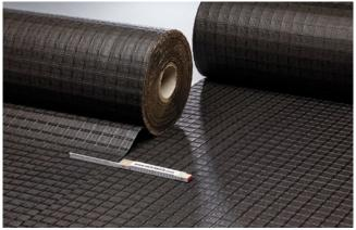
In the cross direction the overlap should be 150 mm. When placing several roll widths side by side the joints should be staggered. The overlaps should be treated with a minimum of 0.15 kg/m<sup>2</sup> of bitumen emulsion.
