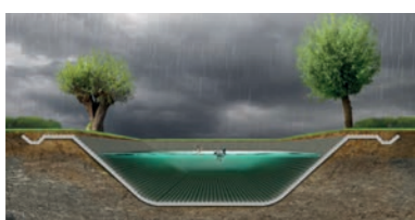
Stormwater holding and storage basins
