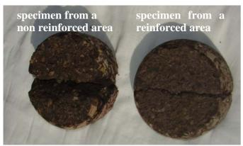
Figure 9. Specimens from areas with (right) and without (left) reinforcement.
